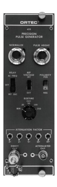
The ORTEC Model 419 is a Precision Pulse Generator that simulates the detection of a nuclear particle reaction in a semiconductor or scintillation detector, as well as serving as a specialized pulse generator for use with pulse processing instrumentation. It can be calibrated to read directly in terms of equivalent energy deposition in semiconductors, and the rise time of the pulse may be varied to simulate the collection time constant in the detector.
