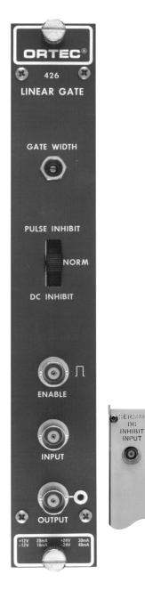
The ORTEC Model 426 Linear Gate provides a variable gate duration with width controlled by a single-turn front-panel-mounted potentiometer. The nominal gate duration is from 0.3 to 4  $\mu$ s. Operation of the linear gate is controlled by a positive enable pulse. It is useful for selecting or inhibiting linear signals according to chosen coincidence or timing requirements.
