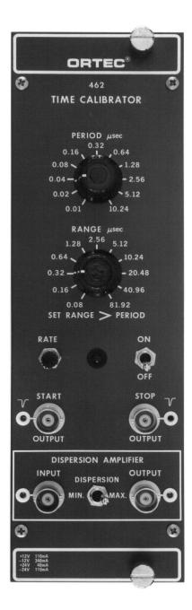
Fast, easy calibration of timing equipment such as time-to-amplitude converters is a routine operation with the ORTEC Model 462 Time Calibrator. The start and stop pulses from the Model 462 are separated by an integral multiple of a precise time period that can be selected by the operator. The accuracy of this time period is  $\pm 10$  ps for a 10-ns period and is  $\pm 0.005\%$  of the total period for longer periods. The long-term stability of this signal is better than 100 ppm.
