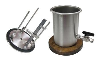
pump does not have to be turned off while the samples are being changed. A quarter turn of the valve opens the chamber to vacuum while sealing off the vent passage.
