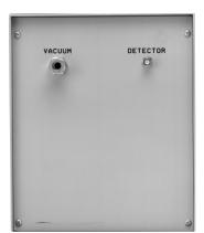
The ORTEC Model 808 Vacuum Chamber provides a quick and convenient way to measure the alpha and beta activity of environmental samples. It accommodates a wide range of sizes of samples and detectors. The chamber can accept sample trays measuring up to 10.8 x 14 cm (4.25 x 5.5 in.), with nominal sample size 10 cm (4 in.) in diameter.
