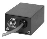
The ORTEC Model 9301 low-noise, fast-rise-time Preamplifier has been designed for use with photomultipliers, electron multipliers, and other detectors employed in photon counting, ion counting, or fast-timing applications. When connected to the detector, the  $50-\Omega$  input resistance of the Model 9301 provides a load resistance for the detector output current pulse.
