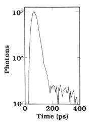
Figure 1. The Fluorescence Lifetime Instrument Response Function Recorded with a Model 9306 1-GHz Preamplifier and the Model 9307 pico-TIMING Discriminator. Time resolutions from 30 to 60 ps FWHM are possible with the system shown in Figure 2.
