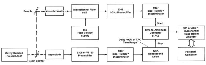
Figure 2. Typical Block Diagram for a Fluorescence Lifetime Spectrometer.
