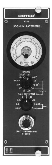
Designed for photon or ion beam applications, the ORTEC Model 9349 Log/Lin Ratemeter provides two modes of operation: linear and logarithmic. The linear mode has 11 full-scale ranges from 10 to 10° counts/s in 1-3-10 steps. The 5-decade log mode covers the range 10 to 10° counts/s in a single span. These choices permit optimum measurement of low, medium, or high steady pulse rates or monitoring of rates that vary through a wide range.
