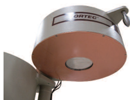
Figure 6. Pancake detector mounted into top door of shield.
