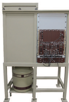
Figure 2. Analog Compton Suppression System
