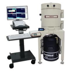
DSPEC LF is a member of the DSPEC USB family of digital technology gamma-ray spectrometers from ORTEC. It provides the same rock solid spectral stability with variation in temperature and count rate and retains many of the valuable attributes of the other two models. Many environmental and radiochemistry laboratories will find this instrument to be the best MCA for day-to-day sample counting with laboratory HPGe or NaI detector systems.
