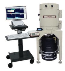
DSPEC LF is a member of the DSPEC USB family of digital technology gamma-ray spectrometers from ORTEC. It provides the same rock solid spectral stability with variation in temperature and count rate and retains many of the valuable attributes of the other two models. Many environmental and radiochemistry laboratories will find this instrument to be the best MCA for day-to-day sample counting with laboratory HPGe or NaI detector systems.
