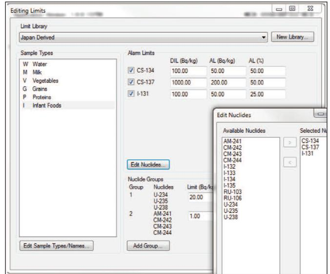
The ORTEC FoodGuard-2 workstation is a ready-to-use, full featured system for performing sophisticated analysis of food, water, and other agricultural samples containing any form of gamma ray emitting radioactive material which can be present following an accident or terrorist incident. By the use of a high-resolution, high-purity germanium (HPGe) detector, each and every gamma ray emitting radionuclide in the sample is quantified in terms of specific activity in Bq/kg or Bq/liter.
