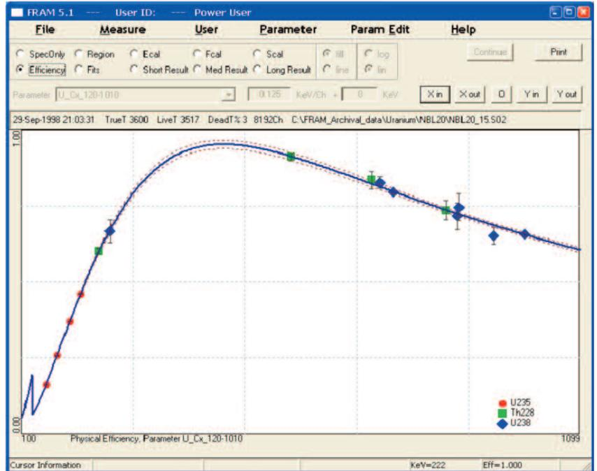
A relative efficiency curve plot from the analysis of a coaxial detector spectrum from 200 g of  $U^{308}$  enriched to 20%  $^{235}U$ .
