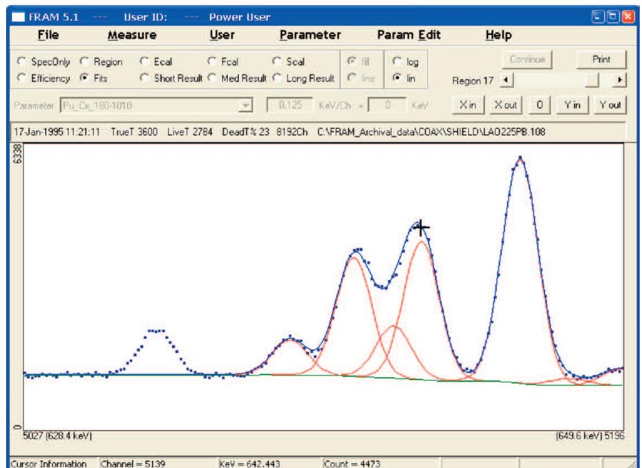
Fitting in the 640 keV region from the spectrum of a 1 kg PuO<sub>2</sub> sample with 16%  $^{240}\text{Pu}$ .
