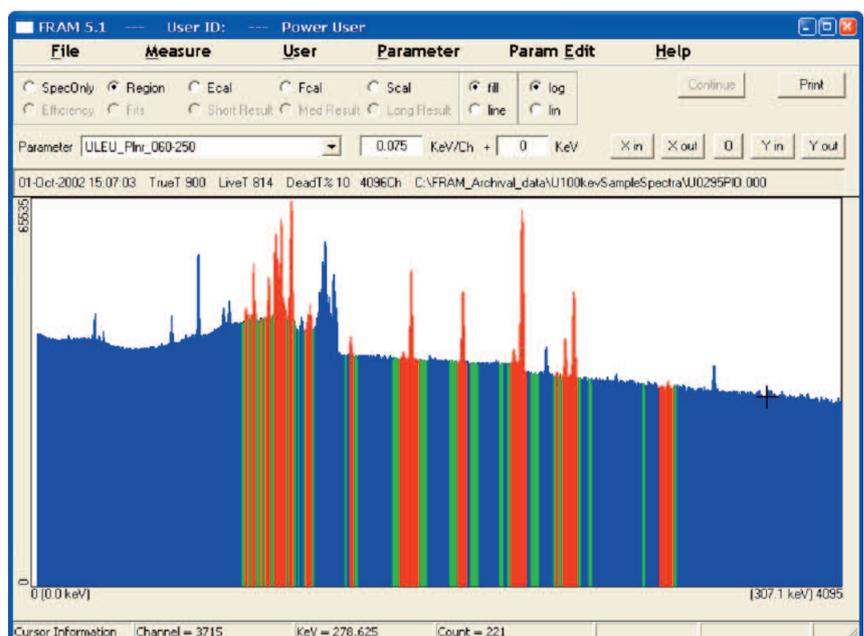
The highly graphical FRAM user interface complies with the latest Windows conventions and is easy to use. A single interface is provided for all data displays. A single dialog bar controls all aspects of spectrum and results display, making it easy for the user to verify the quality of the data or analysis without leaving the FRAM main window.
