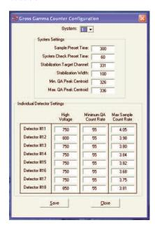
The sample screening software application manages the system ensuring reliable and simple operation. Setup is very simple; a single parameter entry screen sets the 8 detector bias settings, the stabilization and threshold limits and a common acquisition preset for the sample batches to be screened.
