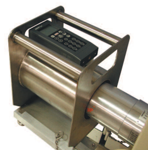
ISO-LASERMETER mounted on SHD-1.
