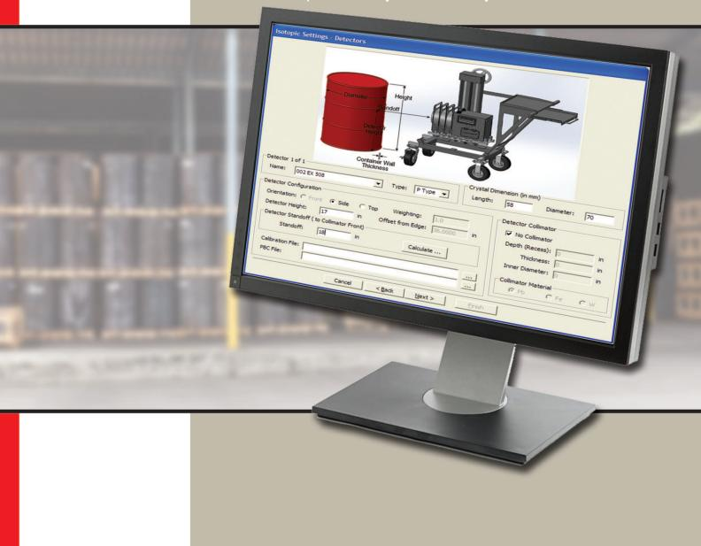
ISOTOPIC provides an integrated, practical solution to a wide range of gamma-ray measurement problems encountered in radioactive waste assay and characterization applications. High resolution, high purity germanium (HPGe) spectra are analyzed and assay results determined for large-scale bulk samples.
