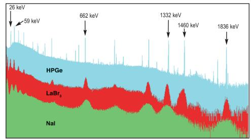
Figure 1. Comparison for LaBr<sub>3</sub>(Ce), NaI(TI), and HPGe spectra.
