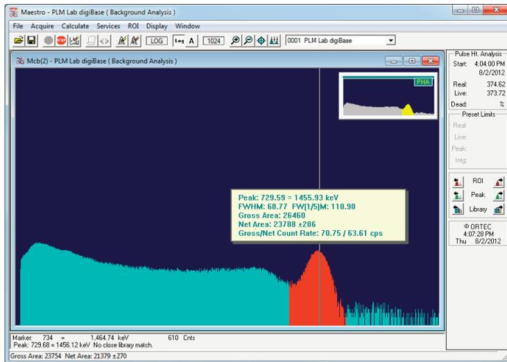
When viewing a live detector, the spectrum view is updated in real time and provides current spectral data, live peak calculations, and hardware properties — even for remote instruments connected to different computers on the network. Viewing spectrum peaks, library energies, or regions of interest is simple with the convenient side panel buttons.
