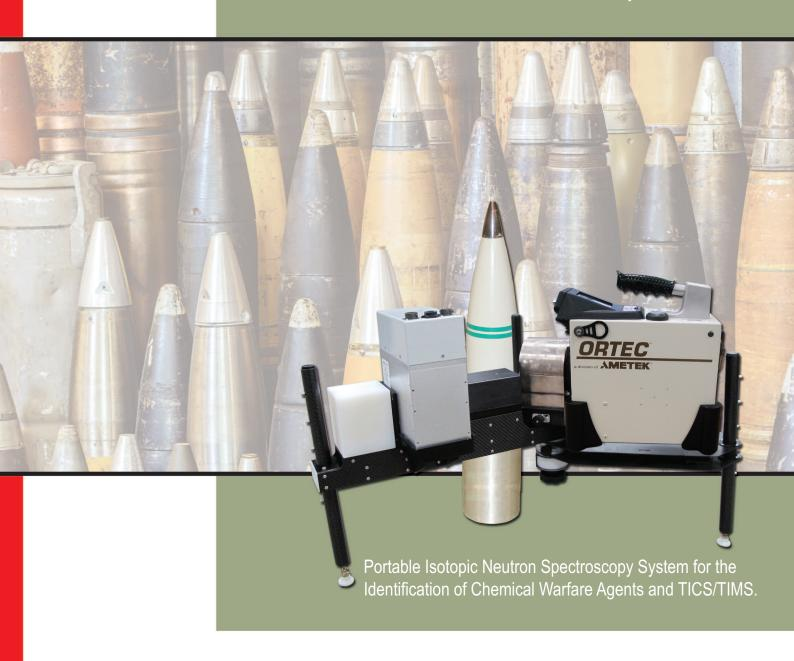
Working with the U.S. Department of Defense and Idaho National Labs, ORTEC has developed the PINS3-CW-G2 Portable Isotopic Neutron Spectroscopy (PINS) Non-Destructive Assay System. This new system is lighter, more portable, easier to set up, and easier to deploy on missions.
