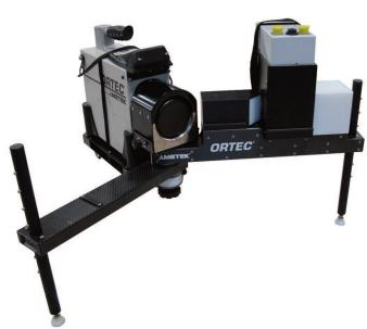
The PINS3-CW-G2 incorporates the miniGEN D-D Neutron Generator which is approximately 66% smaller, 66% lighter, and uses 60% less power than the previous generator.
