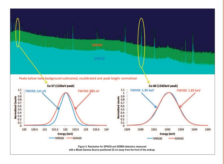
Better resolution performance of PROFILE "SP" Series detectors translates into an improved Peak to Background ratio, which in turn implies lowered Minimum Detectable Activity (MDA) and/or shorter counting times.
