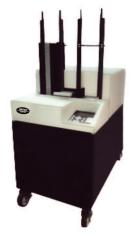
The WPC-1150-GFW-3.5 and WPC-1150-GFW-5 low background automatics are gas-flow proportional counters equipped with either a 3.5 in. (8.9 cm) or 5.0 in. (12.7 cm) detector configuration. Each counter incorporates a built-in color touch screen interface and is targeted toward Health Physics and environmental applications. They are ideal for large diameter air filters used in high-volume air samplers.
