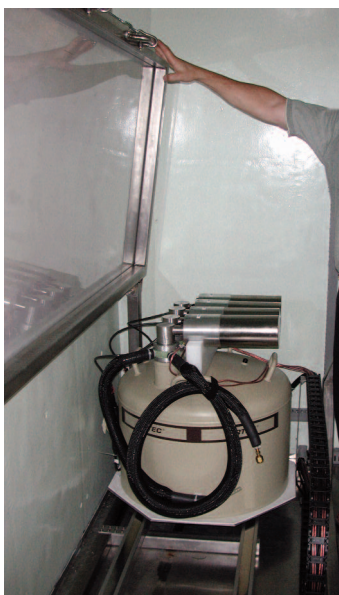
LN 2 based Detectors in Scanning Whole-Body Counter (mounted under bed).
