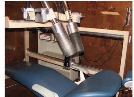
Low-Background Room with Whole-Body Counting Detectors Cooled with Mechanical Coolers.
