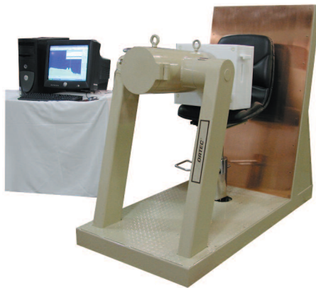
Nal System with Single, Large Crystal in Collimated Shield and Swivel Seat.
