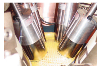
Four Detector ACTINIDE-85 Array for Lung Burden Measurements.
