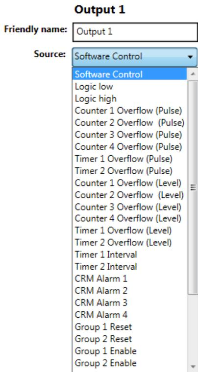
Figure 16. Output Setup.
