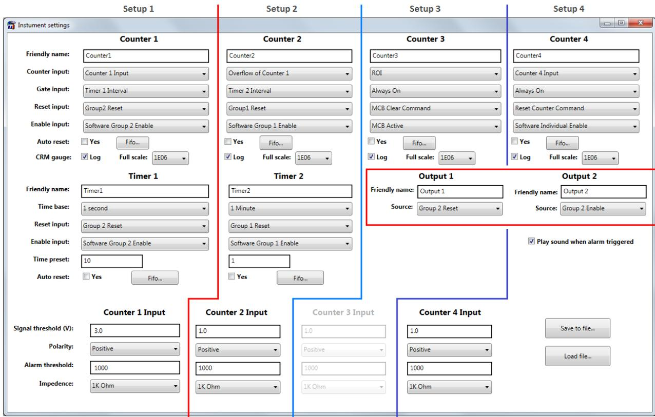
Figure 25. The First 928 Configured for Four Tasks.
