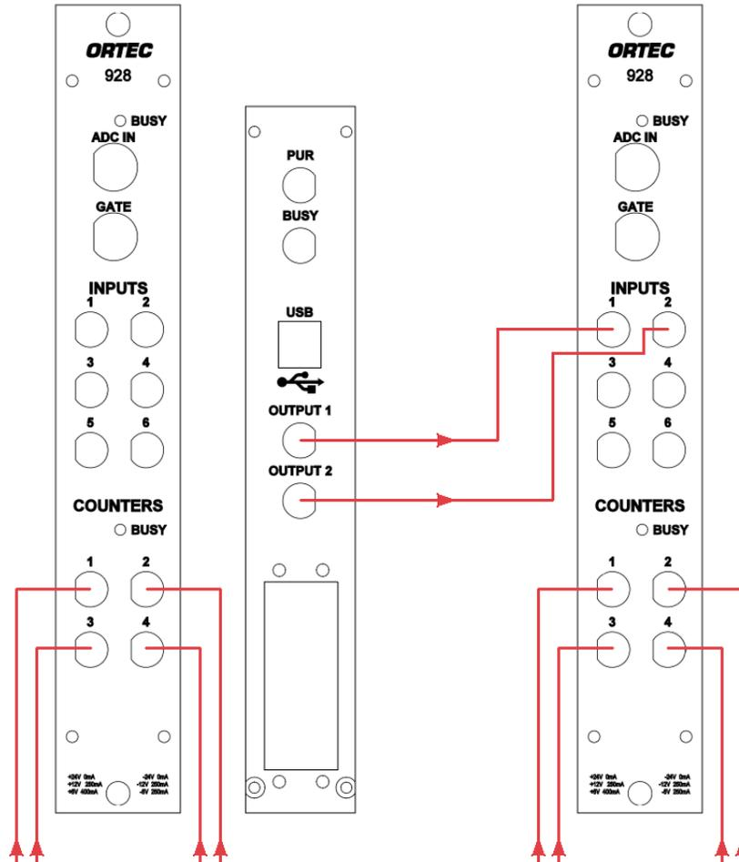
**Figure 22. Cabling Eight Counters To Run From One Timer.**
