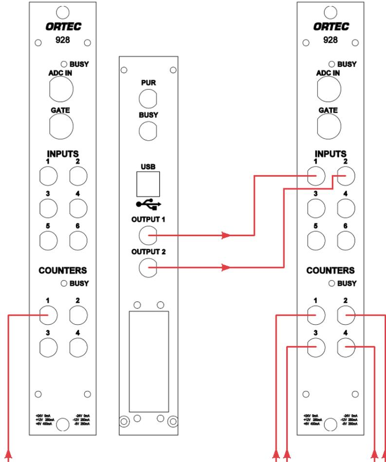
Figure 26. Task 1: Cabling Counter/Timer Group 2 To Control a Second 928.
