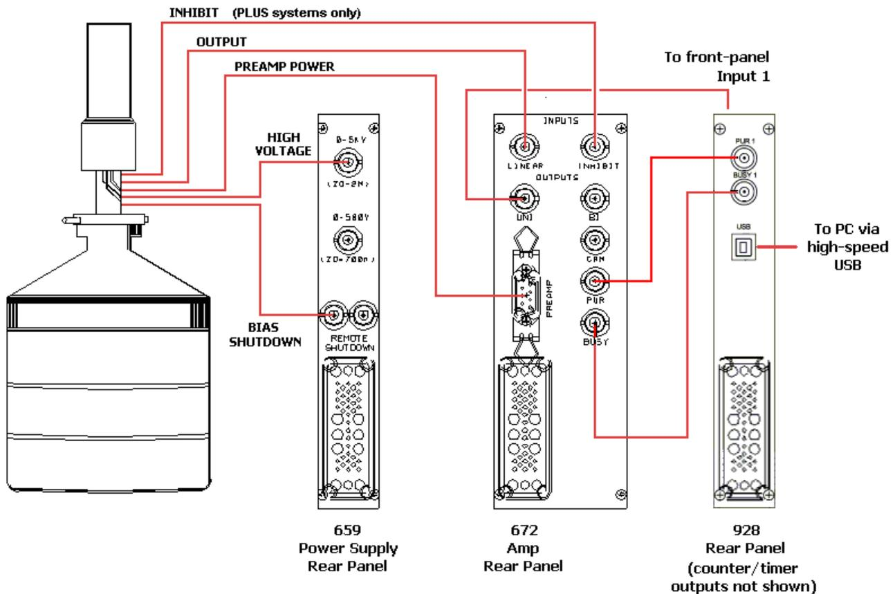
Figure 4. HPGe System Cabling (928-MCB rear panel [no outputs] pictured for clarity).
