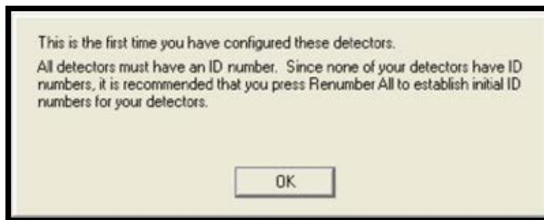
Figure 25. New Instruments Must Have a Non-Zero ID Number
