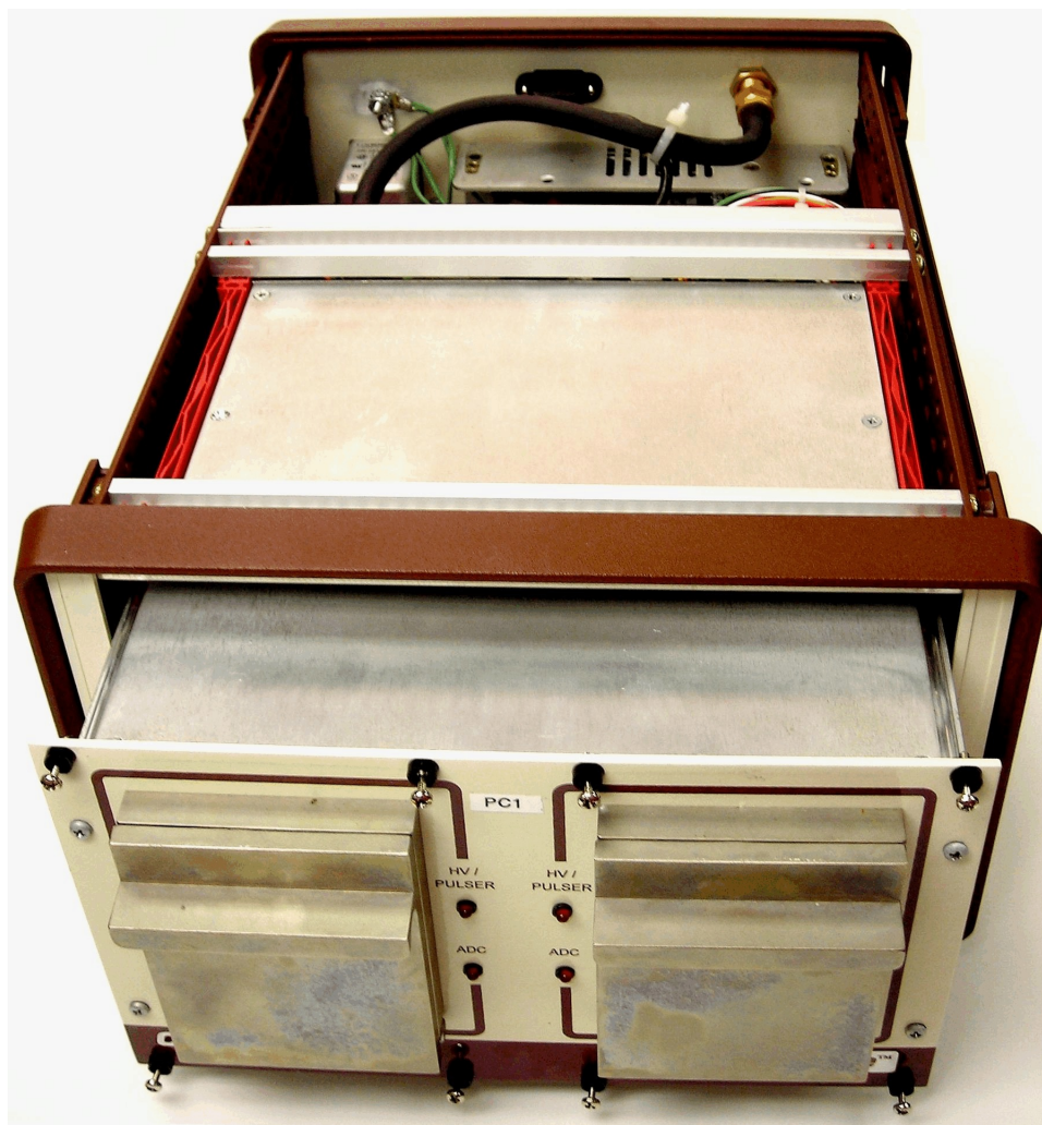
Fig. 14. Alpha Duo Partially Removed from Benchtop Enclosure
