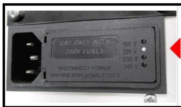
Figure 27. Note Position of Voltage Indicator Pin
