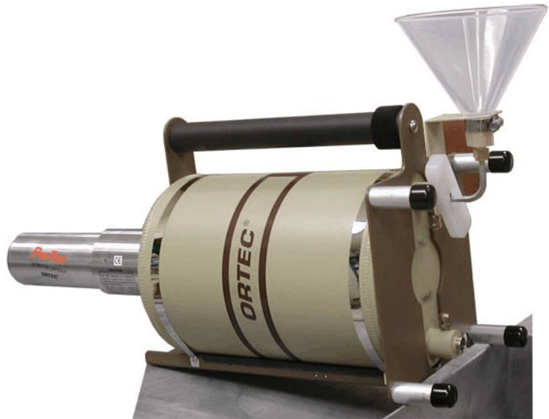
Fig. 9. Slightly Elevate the Bottom of MOD Dewars for Easier Filling.
