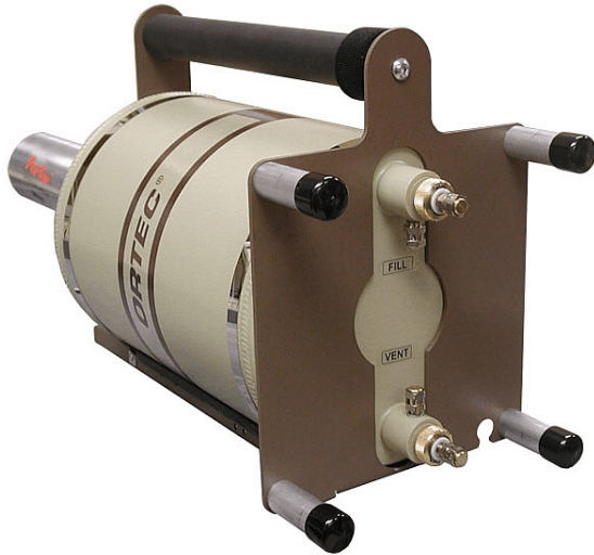
Fig. 1. MOD Dewar (showing FILL and VENT tubes).
