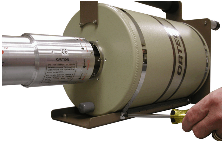
Fig. 6. Unscrewing the Metal Straps.
