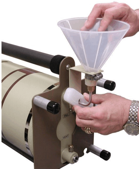
Fig. 8. Fill Funnel Assembly (showing MOD dewar, fill tube inserted, plastic nut being tightened on FILL tube neck threads).
