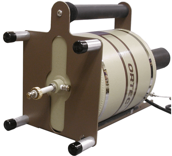
Fig. 2. All-Attitude Dewar (showing FILL/VENT tube with plug partially removed).
