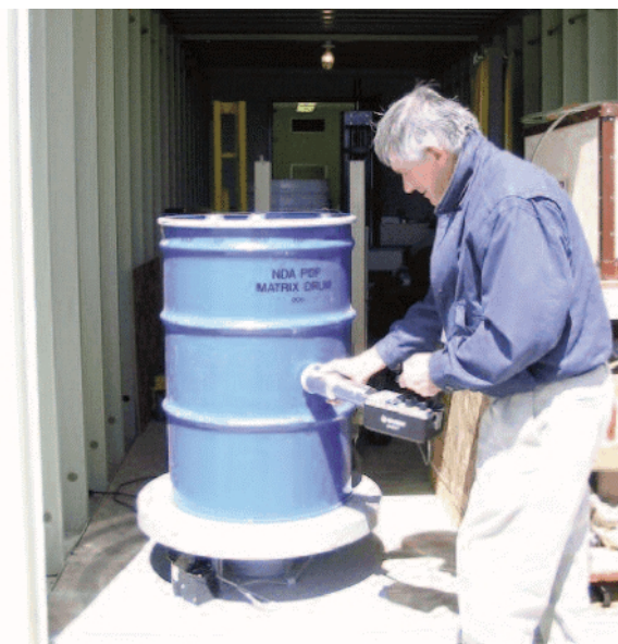
Figure 60. Scanning for a “Hot Spot.”
