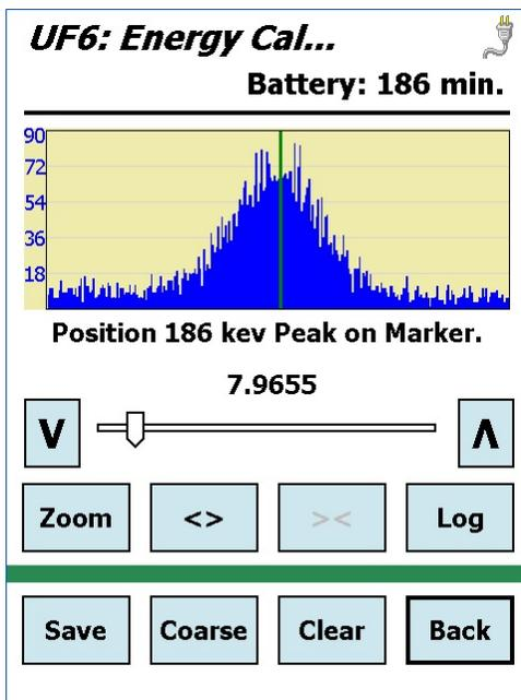
**Figure 34.** Adjust the Fine Gain to Center the 185.7 keV Peak in Channel 2476.
