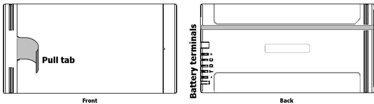
**Figure 71.** Front and Back of Internal Battery.
