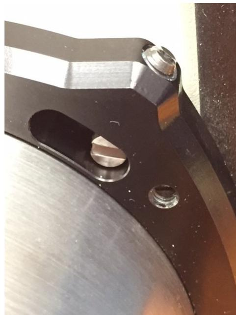
**Figure 10.** Collimator Locked.
