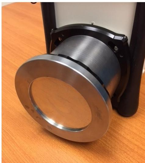
**Figure 14.** Tin Filter Attached.
