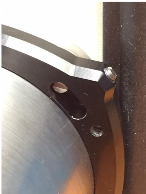
**Figure 9.** Collimator Unlocked.
