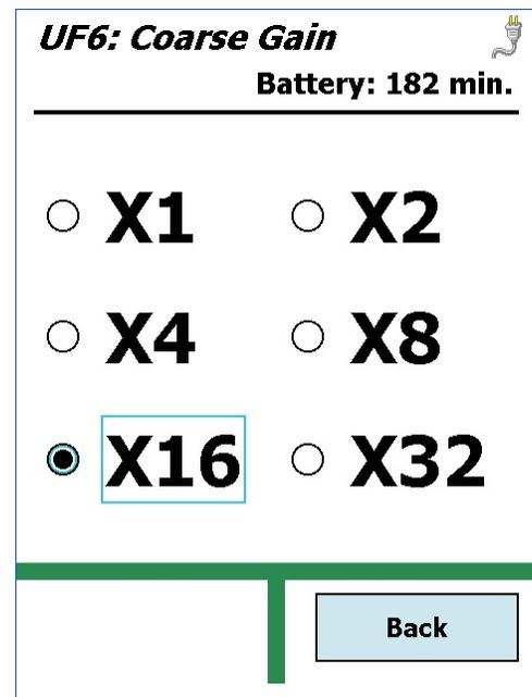
**Figure 35.** Amplifier Coarse Gain Settings.
