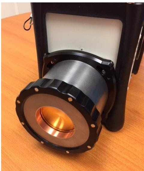
**Figure 12.** Collimator with Open End Cap.
