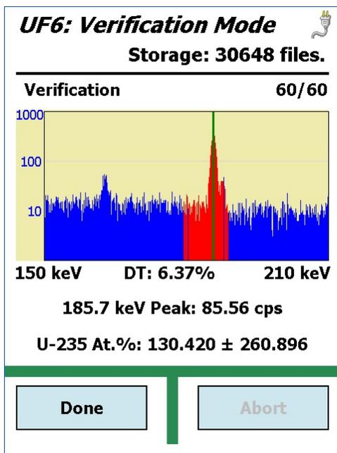
**Figure 50.** Spectrum and Enrichment Data for Completed Verification.
