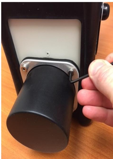
**Figure 4.** Dust Cover Bolt Removal.
