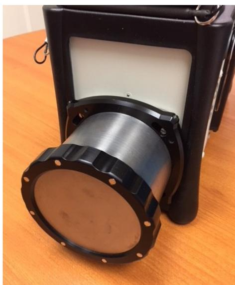
**Figure 13.** Collimator with Full End Cap.
