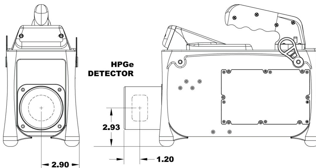
**Figure 61.** Reference Points for the HPGe Detector (all measurements in inches).
