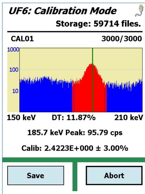
**Figure 46.** Spectrum and Calibration Constants for Completed Calibration Acquisition.
