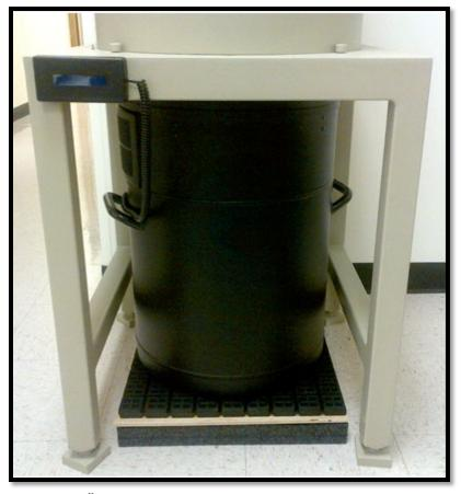
Figure 11. The MÖBIUS Installed on Foam, Plywood, and Anti-Vibration Pad
