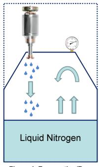
Figure 1. Evaporation/Re-Condensation Process
