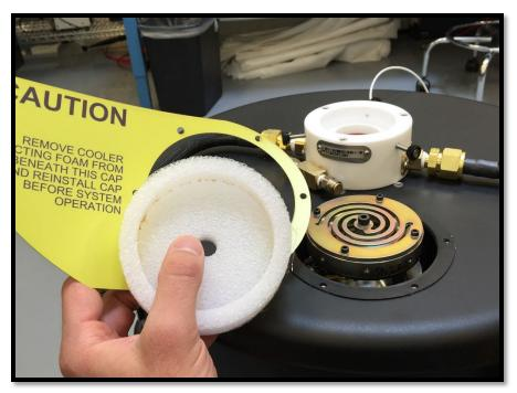
Figure 6. MÖBIUS with Protective Foam Block and Caution Tag Under Cooler Cover Being Removed
