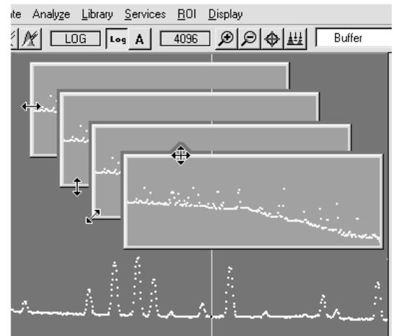
**Figure 38. Two-Sided Pointer for Sizing Full Spectrum View, and Four-Sided Pointer for Moving Window.**
