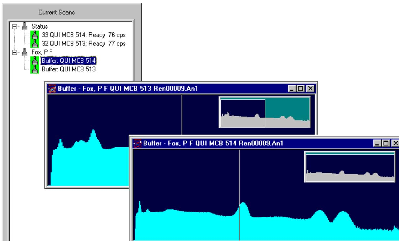
Figure 49. Recalling Individual Spectra from a Multi-Detector Scan.
