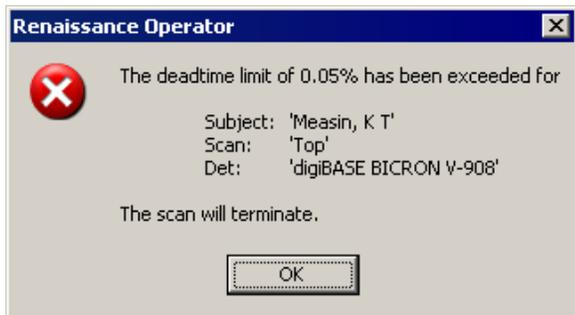
**Figure 4. Count Terminated Due to High Dead Time.**
