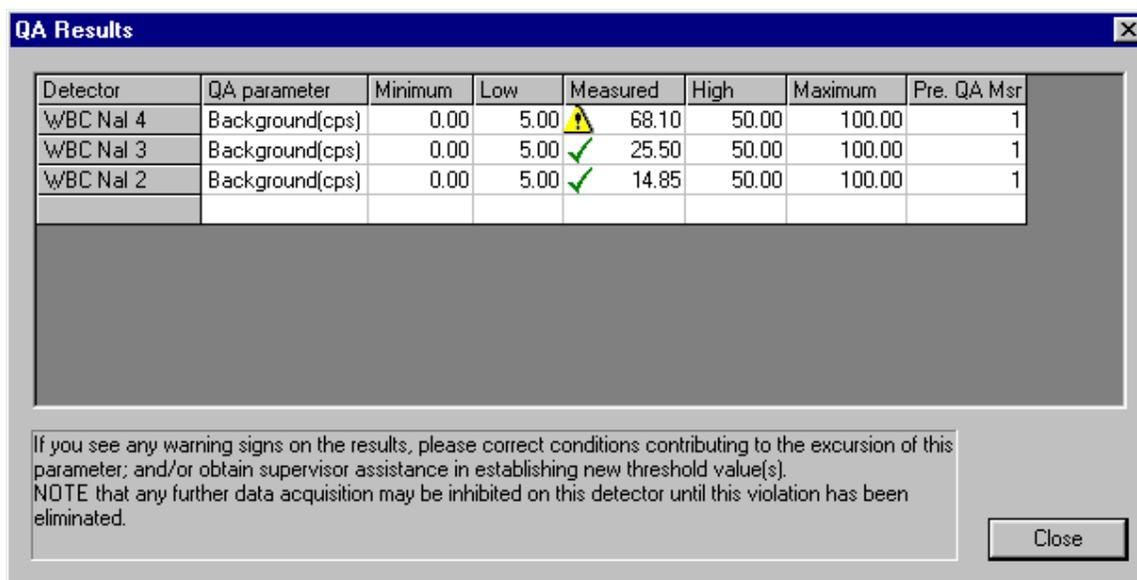
**Figure 19. Background Measurement Results (showing two measurements within limits and one warning).**
