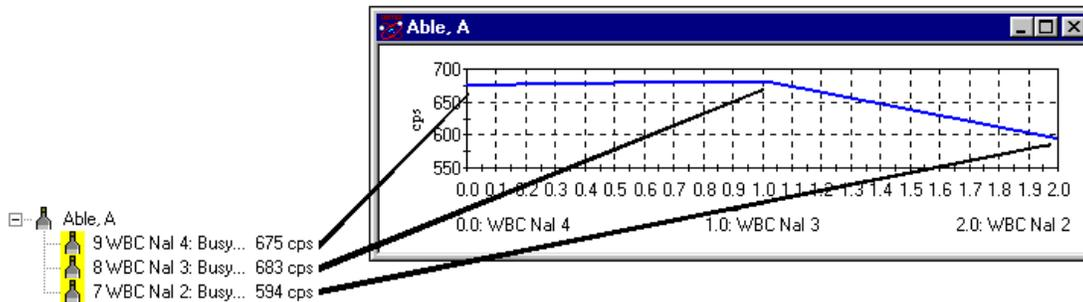
**Figure 26. Summed Spectrum and MCS Windows for Multi-Detector Groups. Note the “At-a-Glance” Display of Input Count Rates for the Detectors in the Group.**
