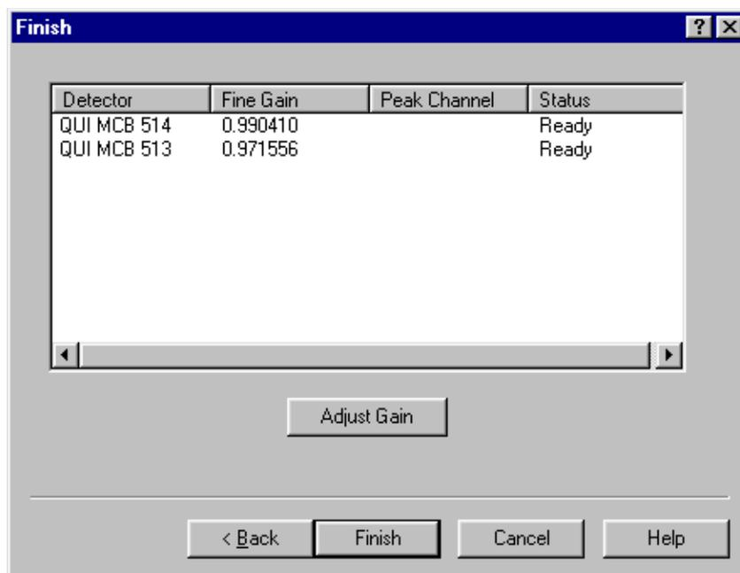
**Figure 14. Gain Adjust Complete (note the new fine gain values).**
