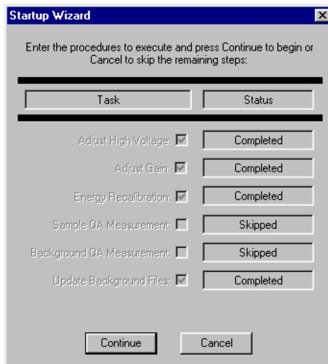
**Figure 22. Startup Completed (note tasks that have been completed or skipped).**
