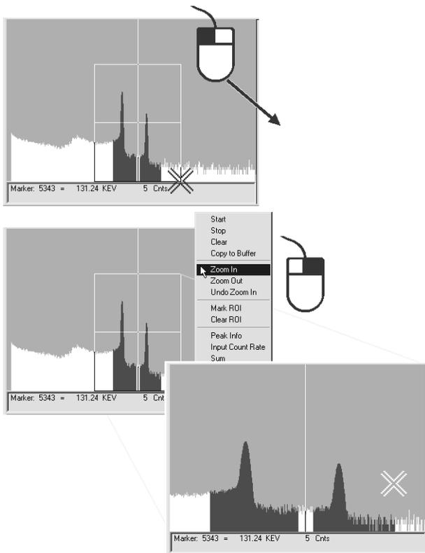
**Figure 37. Zooming In Using the Rubber Rectangle and Right-Mouse-Button Menu.**
