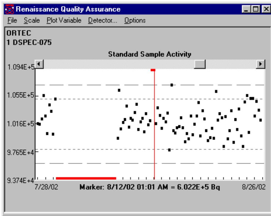
Figure 81. Control Chart On Screen with Fixed Vertical Scale On.
