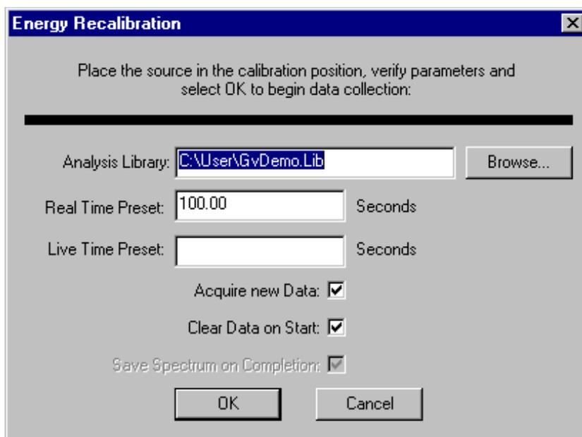
**Figure 15. Start the Energy Recalibration.**
