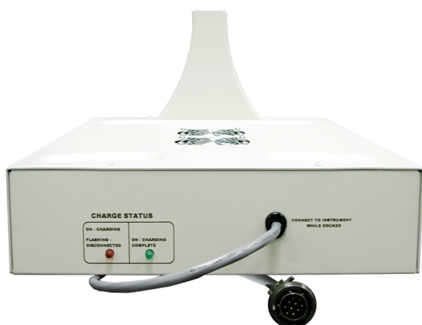
Figure 8. Docking Station Front Panel and Battery Charger Cable.
