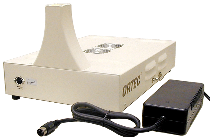
Figure 9. Docking Station Rear Panel and AC/DC Power Adapter.
