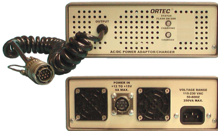
Figure 4. PAC-II Charger, Front and Rear Panels.
