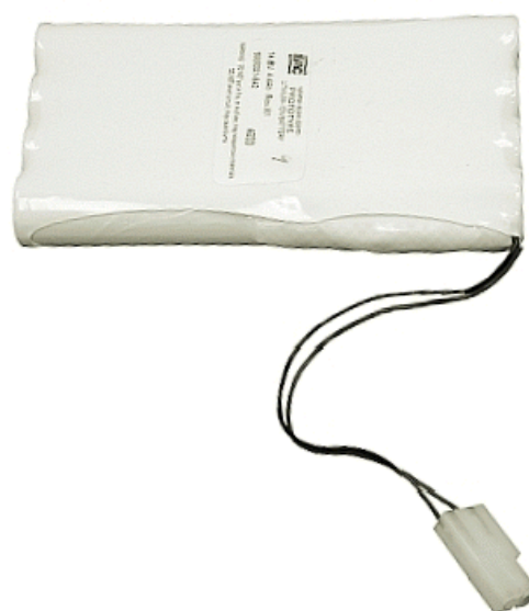
Figure 76. Internal Battery Pack and Connector.
