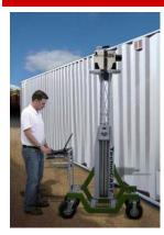
A Convenient Solution to Scanning Large Areas or Containers with the ORTEC Detective Series Hand-Held Nuclide Identifiers
