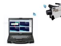
The Mobile MCB Server application offers wireless communication for all Detective and trans-SPEC instruments.
