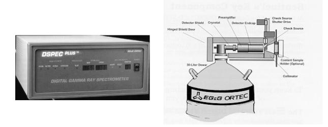
Fig 2. High Purity Germanium (HPGe) detector system with digital signal processing electronics (DSPEC<sup>PLUS</sup>).
