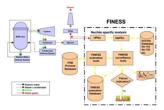
**Fig 1. FINESS** offers instant and reliable fuel failure detection and ability to determine failure type and degradation.
