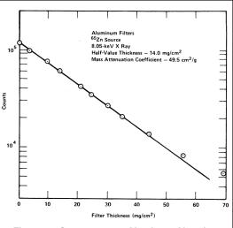
Fig. 11.5. Counts versus Aluminum Absorber Thickness for <sup>65</sup>Zn X Rays.
