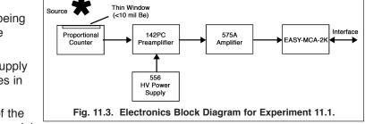
3. Connect the proportional counter to the INPUT of the 142PC Preamplifier using the shortest possible coaxial cable having the appropriate connectors. If the proportional counter employs an MHV connector, the cable will be 75-Ω RG-59A/U with an MHV connector on the end for the proportional counter, and an SHV connector to accommodate the Preamplifier INPUT. If the proportional counter utilizes an SHV connector, the RG 59A/U cable will have SHV connectors on both ends.
