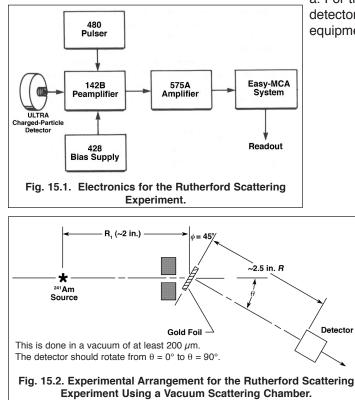
a. For the cable connections between the ULTRA<sup>™</sup> charged-particle detector and the 142B preamplifier, see the description in the list of equipment.
