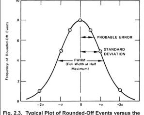
Fig. 2.3. Typical Plot of Rounded-Off Events versus the Rounded-Off Values.
