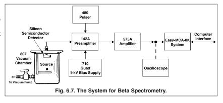
BIAS input on the 142A Preamplifier using the 3.7 m, C-36-12 RG 59A/U 75-Ω Coaxial Cable with SHV Plugs. On the 710 turn the MASTER switch OFF and set all 4 of the 1 kV/100 V/DISABLE switches to DISABLE. Turn all VOLTAGE dials to their minimum value (fully counter-clockwise).
